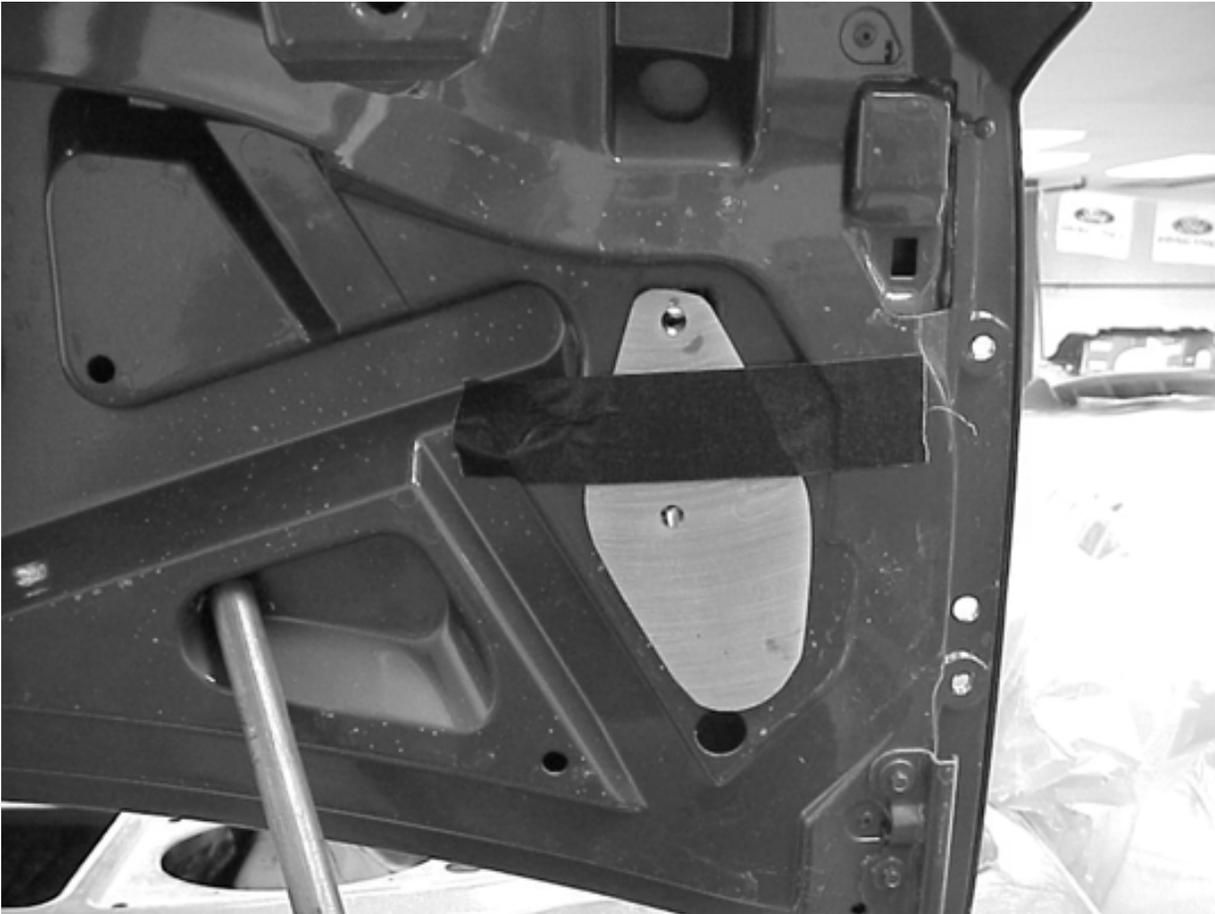
**STEP 3:** Mark the center of each hole with a center punch or marker.
