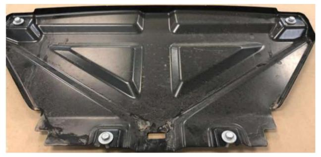
2. If equipped remove lower air dam (12 bolts)
