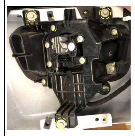
8. Install and secure new FPP/Rigid fog light assembly into bumper facia (torque 28 lb.in)
