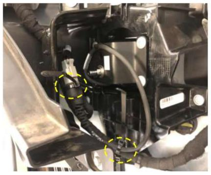
12. Secure excess fog light cable harness length to existing main wiring harness:
