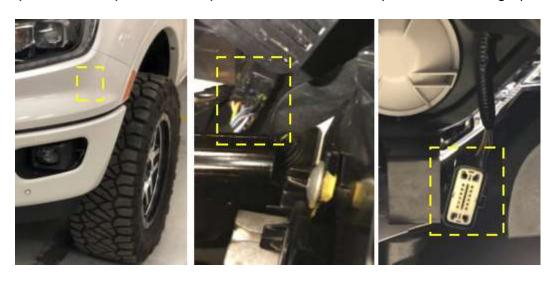
4. Carefully remove 2x fir-tree panel fasteners for main bumper electrical connections at radiator shroud
