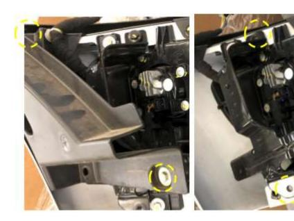
7. Un-couple electrical connection to fog light assembly and carefully remove assembly from bumper facia (3 bolts)
