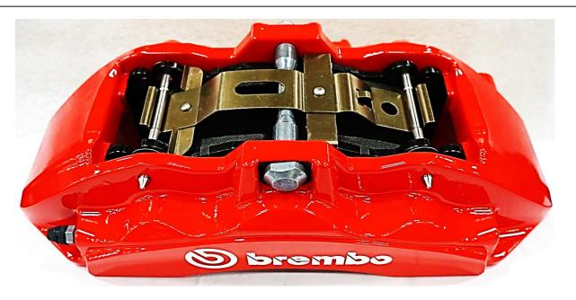
Install the provided Brake Hoses on the Calipers using the provided Banjo Bolts and two (2) Copper Washers per Brake Hose. The Calipers ARE directional. Be sure the Bleeder Screws are pointing up when caliper is installed on vehicle. (*the photo below shows the left Front Caliper*)
