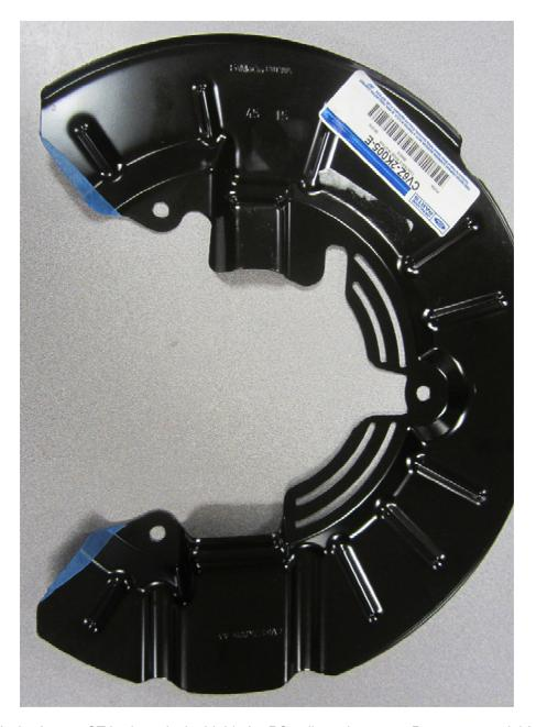
8. Modify the factory ST brake splash shields for RS caliper clearance. Remove material from the blue area. (LH shown)
