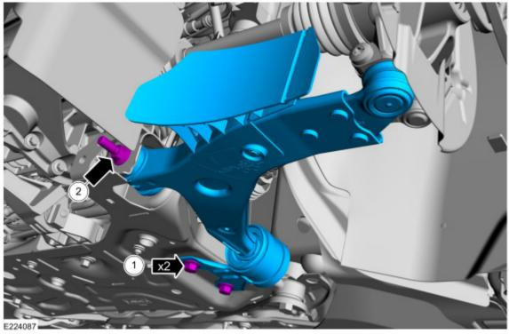
Slide deflectors onto the lower control arm. Install push pins to retain the deflector.
