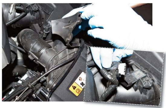
STEP 2: Undo the convoluted hose to crossover duct clip then unfasten the secondary air feed (lower) pipe rubber.
