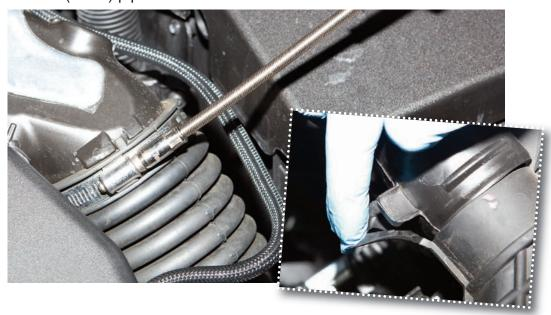
**STEP 3:** Separate the secondary air feed pipe from the airbox - pull apart.
