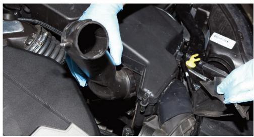
**STEP 4:** The airbox sits on rubber mounts, to remove, pull hard upwards. This will allow access to the shifter arm.
