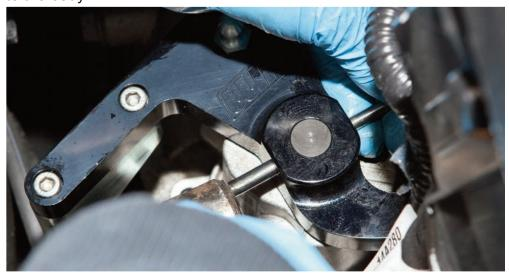
STEP 9: Ensure the roll-pin is fully engaged and that the shifter arm is fixed in postion
