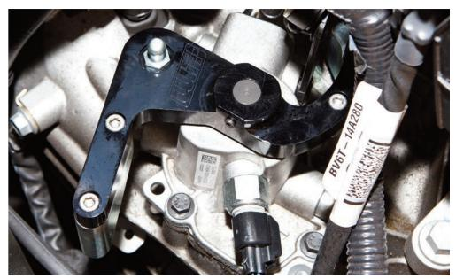
STEP 10: Re-connect both end of the shifter cable as shown below - ensure all gears can be engaged before taking the vehicle for a test drive.
