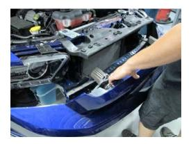
STEP 27: Install the (4) push pins & (4) bolts retaining the upper fascia to the fascia support bracket that were removed in STEP 16. Torque the (4) bolts to 48 in/lb and tighten the (4) push pins.
