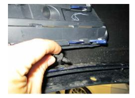
STEP 8: From the backside of the fascia, gently unclip the chin from the fascia by squeezing the tabs. (6) locations.
