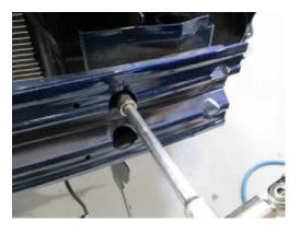
STEP 22: Insert the new splitter bumper bracket from the top side. Hang the bracket from the bumper verifying it aligns over the (2) remaining bumper bolts.
