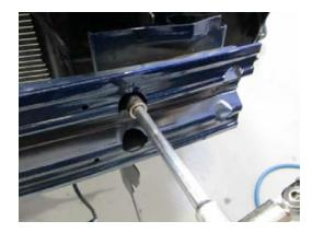
STEP 24: From the backside of the bumper, install the (4) provided bumper nuts and securely tighten onto the newly install splitter bumper bracket, torque to 18 ft/lb.
