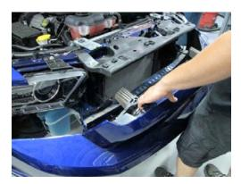
STEP 19: If equipped, unclip both grille fog lamps and remove fascia from vehicle.
