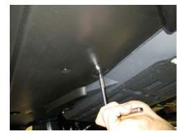
STEP 41: Using the bolts removed in STEP 2, install the (2) outboard bolts and torque to 15 in/lb.
