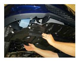
**STEP 5:** Remove the (2) bolts holding the production chin to the fascia.
