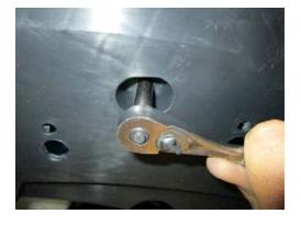
STEP 38: Using the bolts removed in STEP 6, install the (4) bolts to attach the splitters outer edges to the fascia and torque to 15 in/lb.
