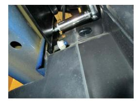
STEP 25: Using the (4) push pins removed in STEP 20, reinstall the impact foam onto the bumper.
