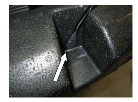
STEP 21: Remove the (2) upper center most bumper bolts.
