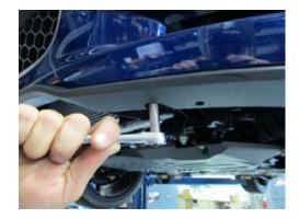
STEP 6: Remove the (4) bolts, (2) per side holding the production chin to the fascia outer edges.
