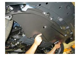
STEP 40: Using the bolts removed in STEP 2, install the (3) rearward bolts and torque to 15 in/lb.
