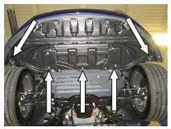
STEP 3: Remove the (12) bolts holding the front edge of belly pan to the fascia.
