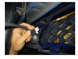
**STEP 11:** From the backside of the fascia, gently unclip the lower grille retaining clips from the fascia (12) locations. Remove the lower grille from the vehicle.
