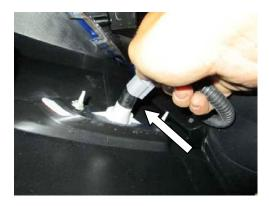
**STEP 14:** Remove the (8) push pins retaining the upper radiator close off shroud.
