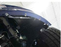
STEP 35: Install the new splitter into the fascia by aligning the splitter clips with the fascia. Gently push into place and verify the (6) splitter clips are securely attached.
