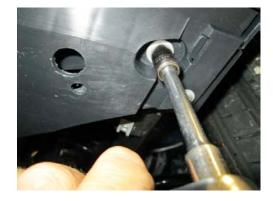
STEP 37 Using the bolts removed in STEP 3, Install (8) bolts into the remaining locations on the new splitter and torque to 28 in/lb.
