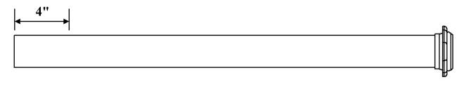
Note: For vehicles with a 122" wheel base, cut 23" off front pipe.
