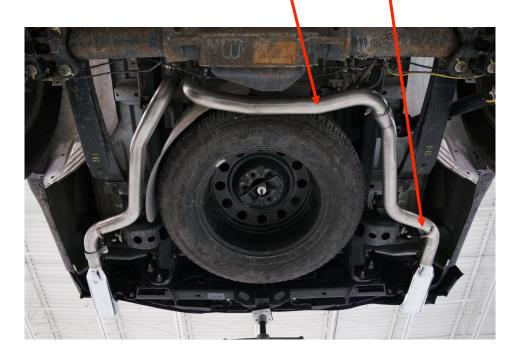
Step 12: Align the right side tailpipe and tip and tighten.
