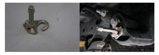
Step 7: Once installed, be sure to torque the shackle bolt to 235 Nm (173 lb-ft).
