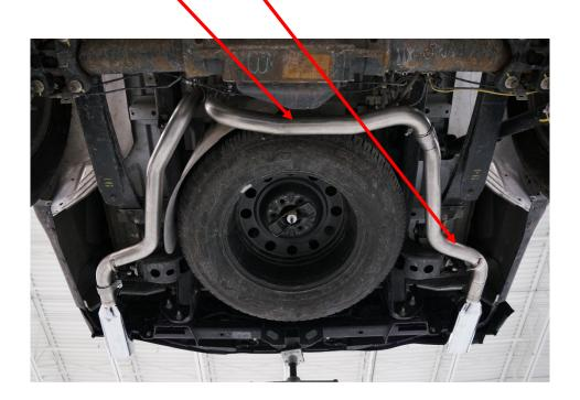
**STEP 11:** Align the right side tail pipe and tip and tighten.
