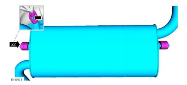
3. Remove 2 rubber hangers from intermediate pipe and remove pipe. (Spray rubber hangers with soap and water to help slide off steel rods.)
