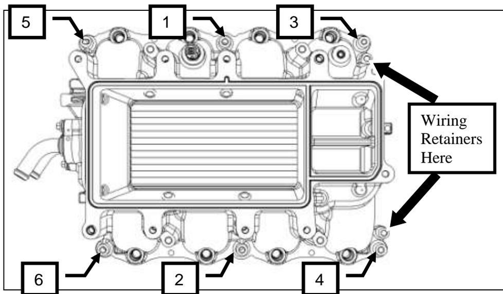
3. Lube the fuel injector o-rings with assembly lube. Install the fuel rail and injectors into the intake manifold using the take off bolts. Be sure each injector is properly seated into the intake manifold. Tighten the bolt pattern in two stages. Stage 1; torque bolts to 10 Nm. Stage 2; tighten bolts an additional 90 degrees.
