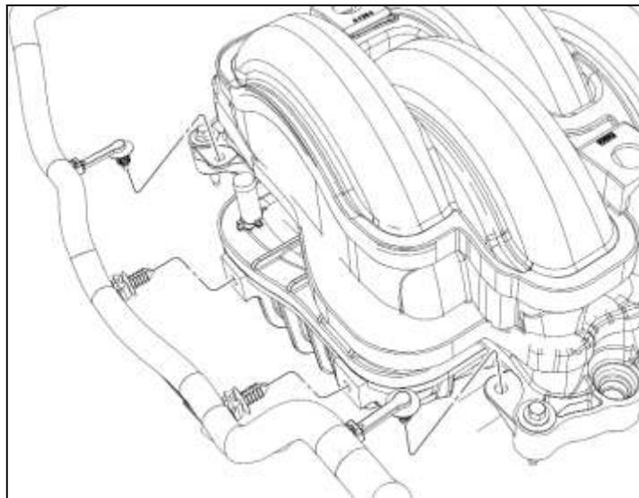
26. Remove and discard the LH and RH fuel rail insulators. Disconnect the (8) fuel injector electrical connectors.
