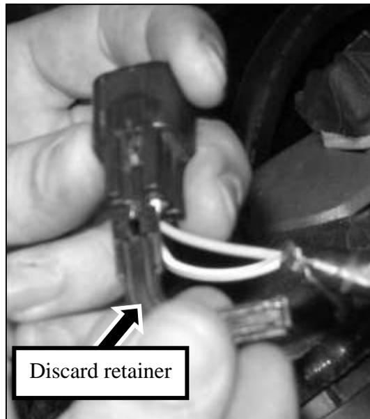
2. Depress the locking tab and separate the “empty” female 1 x 2 connector from the Canister Purge Valve Extension harness (13119G866). This connector replaces the connector removed in the previous step. **Carefully pull the white locking tab forward to allow wires to be installed into the connector.** Populate the new connector such that the white with brown wire is in position 1 and the green wire is in position 2. Depress the white locking tab to secure the wires.
