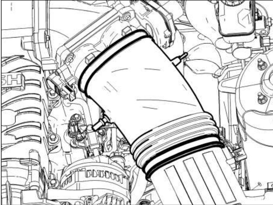
4. Install the PCV Fresh Air Inlet tube (13116758) by connecting the 90 deg fitting to the driver side cam cover and angled fitting to the PCV fitting in the clean air tube.
