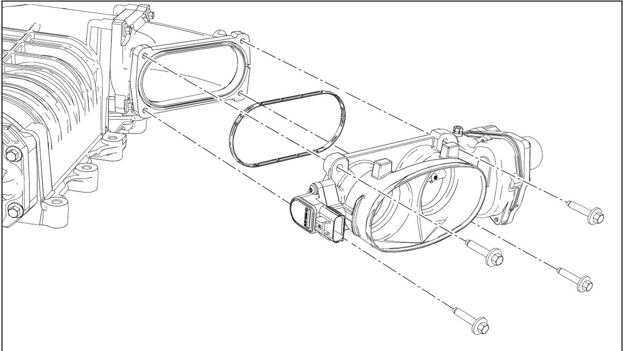
20. Connect the TPS and ETC Throttle Body electrical connectors.
