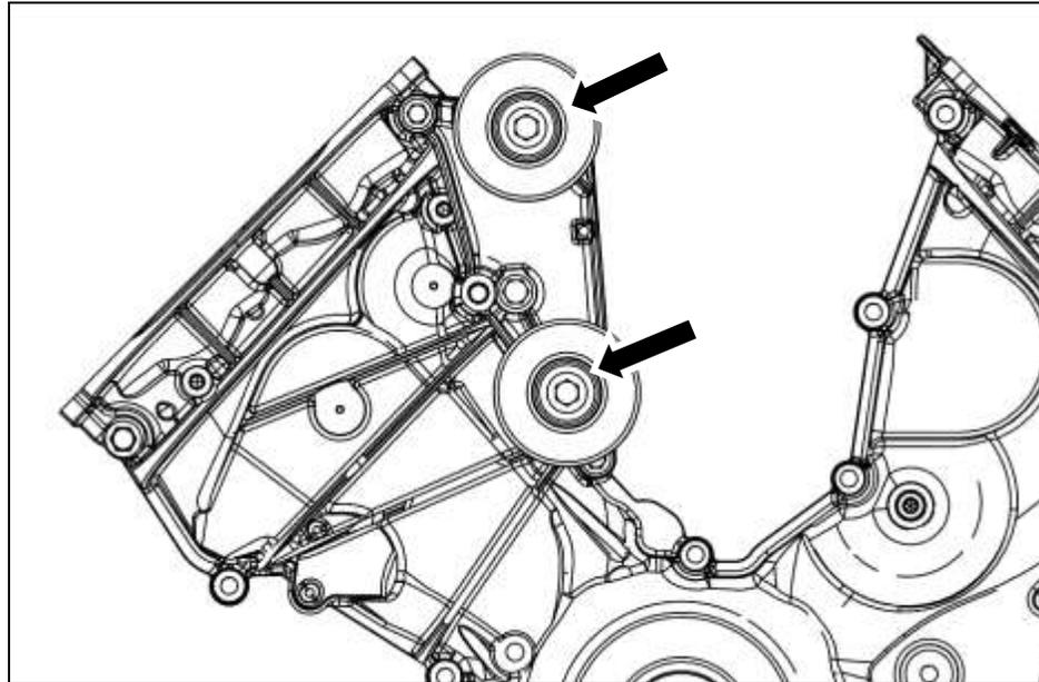
4. Loosely install the FEAD Tensioner Bracket Assembly (13118B603) onto the front cover using (2) M8 x 1.25 x 123mm (R18020055) bolts, leaving atleast a 10mm gap between the two new FEAD brackets.
