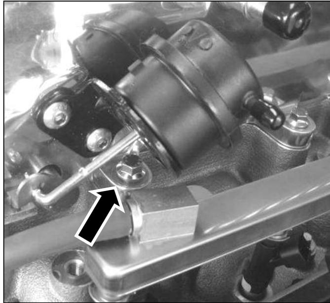
11. Torque the supercharger bolts in an inside-out, criss-cross pattern (sequence: #3-8-2-7-4-9-1-6-5-10). Torque all bolts to 20Nm. Once this is complete, complete a second pass, using the same torque sequence, and torque all bolts to 30Nm.
