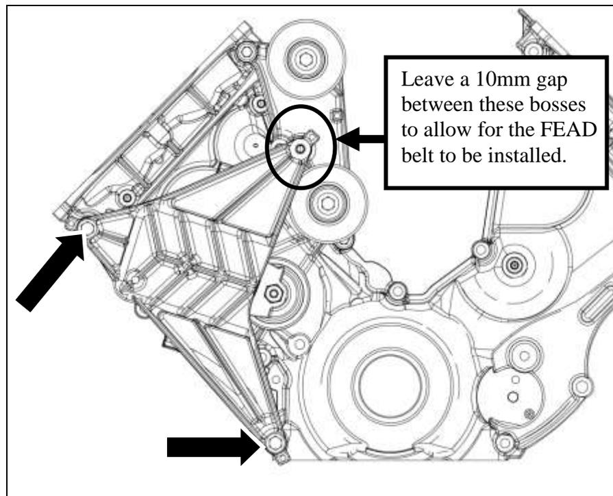
5. Route the FEAD belt (K060825). Do not route the belt onto the supercharger pulley.
