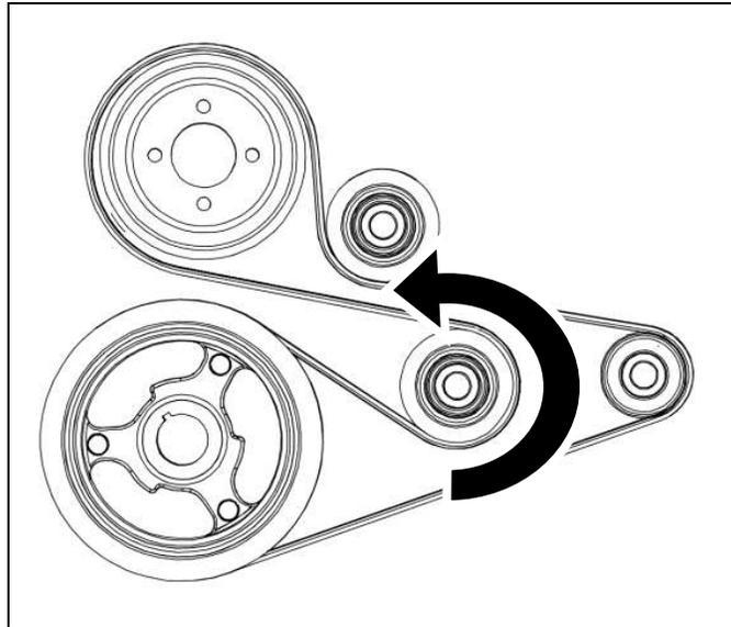
32. Remove the (4) bolts securing the Water Pump Pulley to the engine
