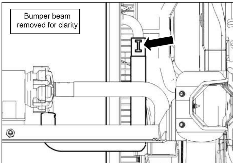
10. Connect the Intercooler Pump Inlet Hose to the inlet port on the intercooler pump. Secure the hose to the pump using (1)  $\frac{3}{4}$ " constant tension clamp. Orient the clamp so the "I" on the hose is in the center of the clamp tangs.
