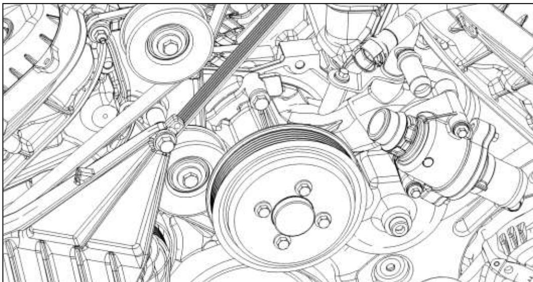
9. Re-install the stock FEAD Belt by rotating the tensioner counter-clockwise and routing the belt as per the stock Ford belt routing.
