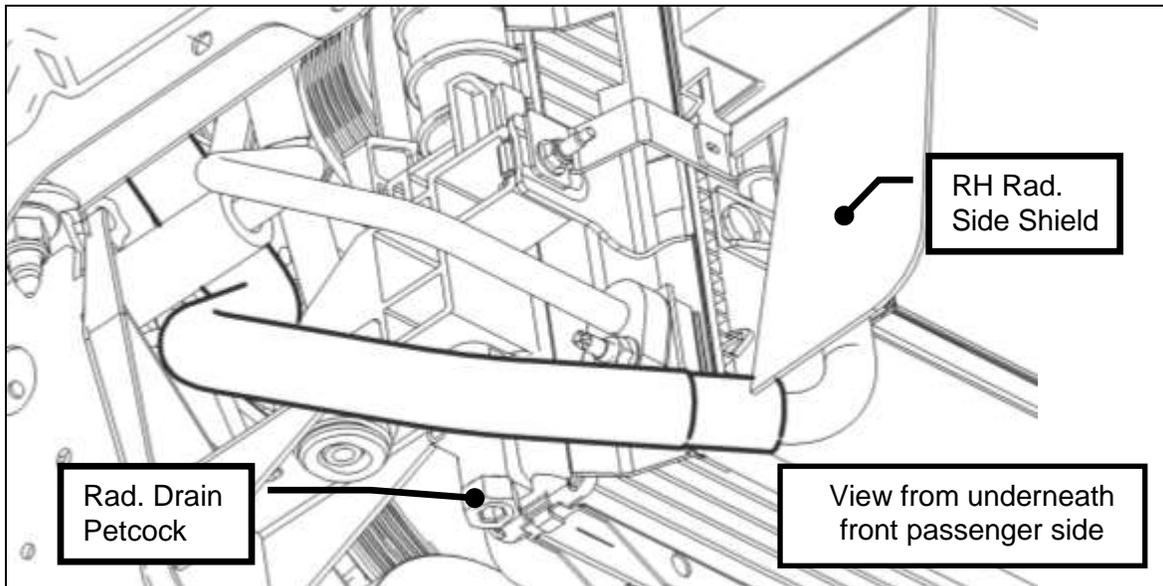
2. Install the Degas Bottle Inlet Hose (13118D031) from the upper intercooler turret to the upper degas bottle fitting using (2)  $\frac{3}{4}$ " constant tension clamps. Orient the clamps so the "I" on the hose is in the center of the clamp tangs.
