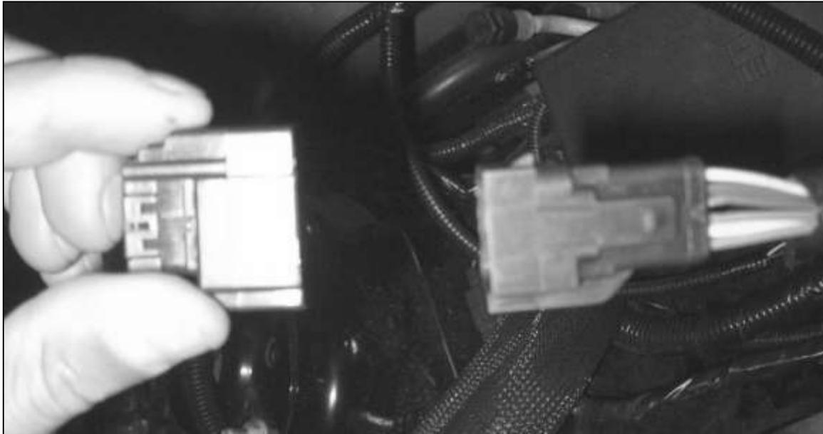
4. Populate the new connector such that the yellow with violet wire is in position 1, the blue with green wire is in position 2, the brown wire is in position 3, the blue with orange wire is in position 4, the yellow wire is in position 5 and the green with violet wire is in position 6. Install the red plastic lock into the connector to secure the wires in place.
