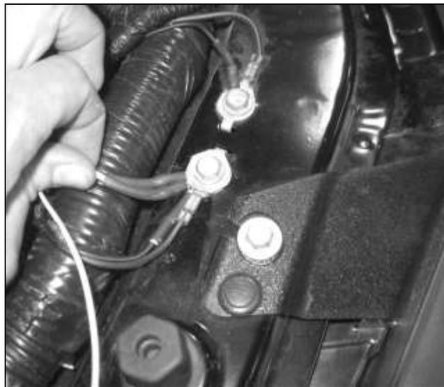
5. Route the single wire with two electrical connectors along the factory engine harness to the rear of the passenger side cylinder head. Connect these two connectors inline with the passenger side radio capacitor. The single connector will be routed to the intercooler pump in Section D of this manual.
