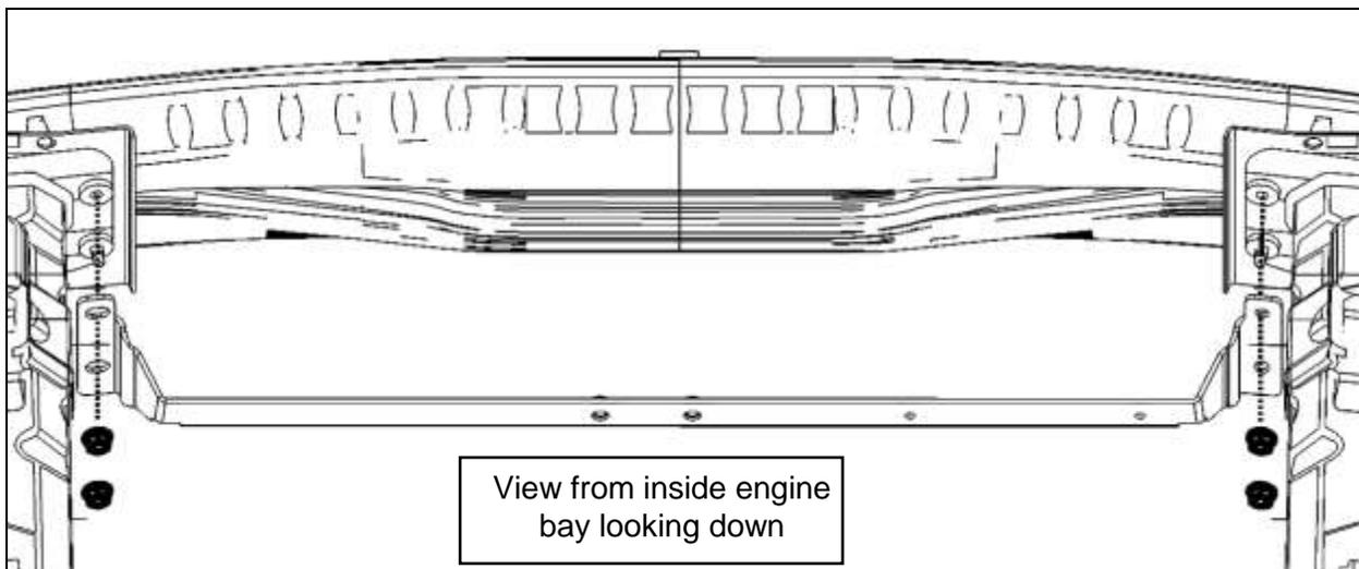
6. Install the Intercooler Pump to Bumper Beam NVH Isolator (13108Z419) on the rear of the bumper beam such that the edge of the pad is 220mm from the driver side bumper beam mounting plate and 60mm from the front edge.
