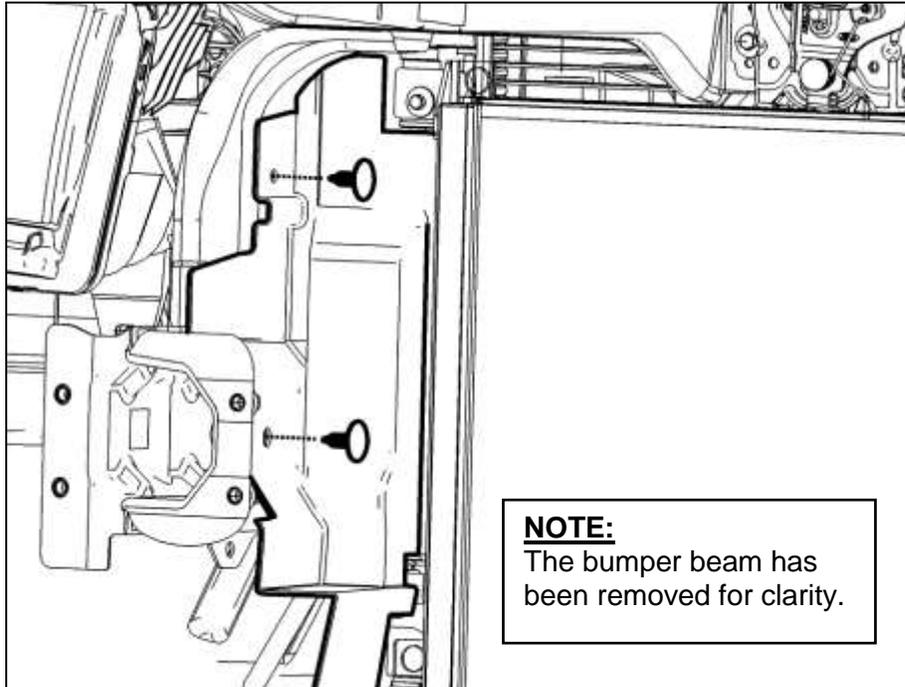
4. Remove the (2) upper, inner front bumper beam bolts.
