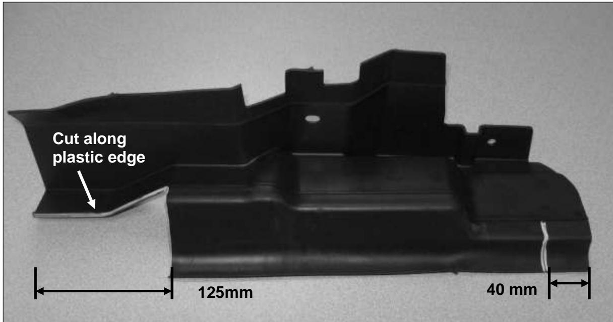
7 - Re-install the RH radiator side shield using the take off push pins.
