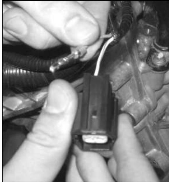
3. Connect the Canister Purge Valve Extension harness to the newly installed connector. The wire colors on each side of the connector pair should align. Route the harness along the main wiring harness to the rear of the driver side cam cover. Use tape or zip ties to secure the extension harness to the main harness.
