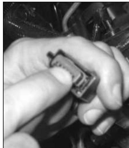
5. Connect the TPS/ETC extension harness to the newly installed connector. The wire colors on each side of the connector pair should align. Route the harness along the main wiring harness to the rear of the driver side cam cover. Use tape or zip ties to secure the extension harness to the main harness.
