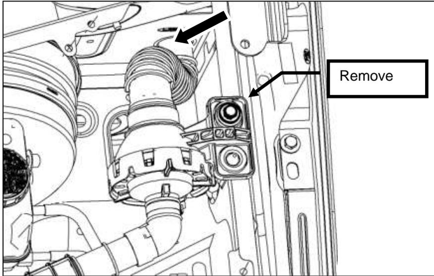
13. Disconnect the PCV Fresh Air Inlet tube from the left-hand cam cover and clean air tube. Remove the clean air tube from the throttle body and airbox. Remove the clean air tube and the induction resonance tube from the vehicle. Neither of these components will be reused.
