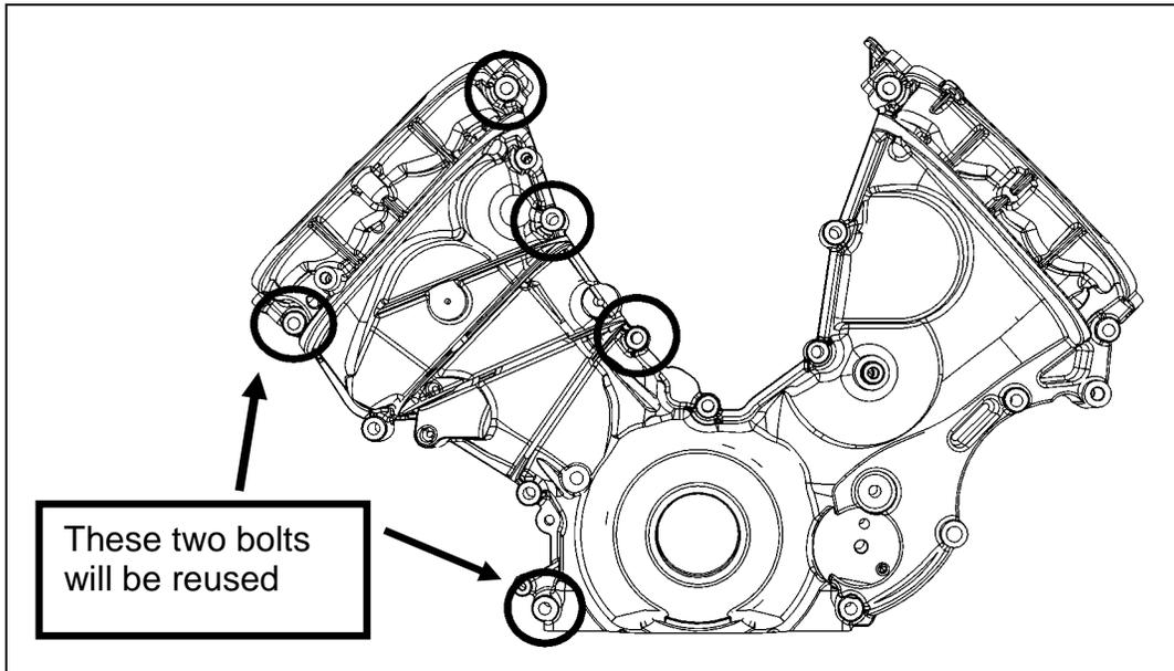
2. Install the Upper FEAD Bracket (13118B653U) using (2) M8 x 1.25 x 57mm bolts that were removed in the previous step and (2) M8 x 1.25 x 84mm bolts (W704752) from Hardware Kit C. Torque bolts to 25 Nm.
