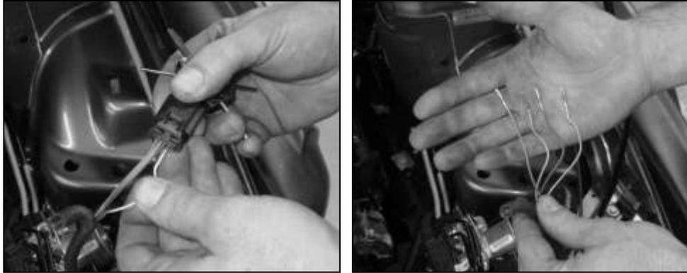
2. Insert the pins from the factory connector into the female connector provided on the end of the MAF Extension Harness (131112B579W). The following color wires go into the following positions on the clip: Violet with Grey – position #2 , Grey with Yellow – position #3, Blue with White – position #4, Yellow with Violet – position #5. NOTE- Positions 1 & 6 are not used.
