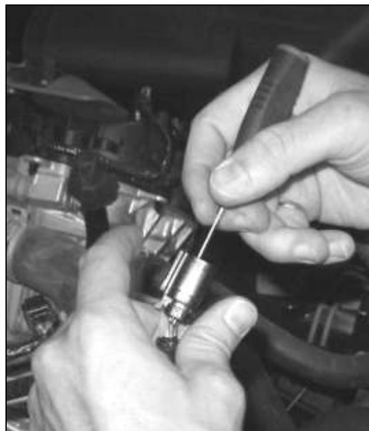
3. Depress the locking tab and separate the “empty” female 1 x 6 connector from the new TPS/ETC Extension harness (131114A595). It will be used in the next step.
