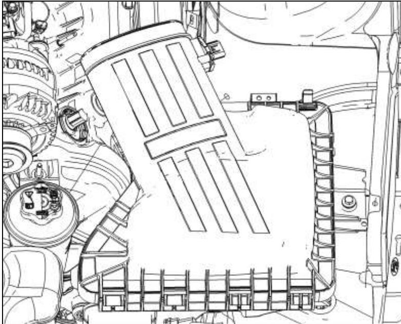
2. Insert the Vacuum Fitting (383004-S) and the ¼" Vacuum Cap (CS515) from Hardware Kit A into the Clean Air Tube (1312-9R504) in the orientation shown.
