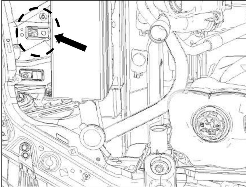
2. Install the relay from the Intercooler Pump Wiring Harness (13118W501) onto the stud. Install the fuse on top of the relay onto the same stud. Use (1) M6 nut (W520412) from the Intercooler Hardware Kit (13116066FRTHKE) to secure the relay and fuse to the stud. Torque the nut to 10 Nm. Reinstall the wiring harness from previous step to the stud for proper retention.
