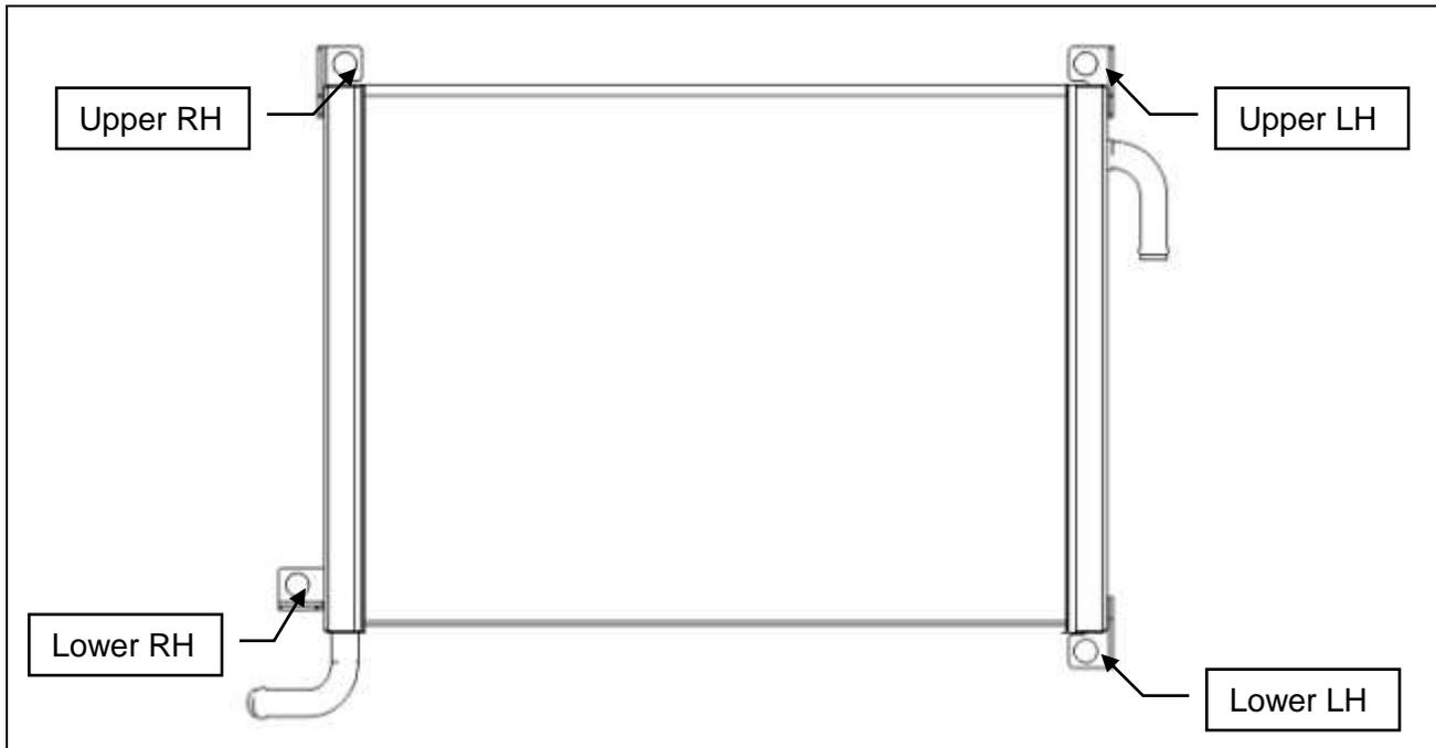
2. Push (1) Sleeve (R07060108) into each of the rubber grommets.
