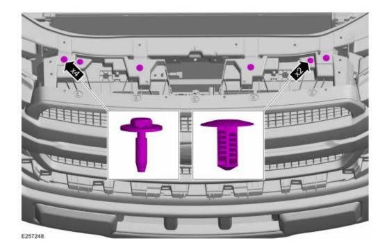
8. Remove the active grille shutter mounting bolts. *Torque*: 159 lb.in (18 Nm)
