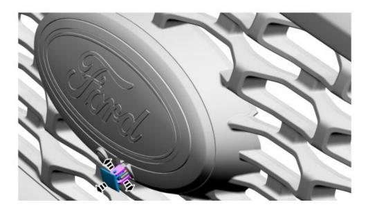
2. Remove the screws and the front camera washer and bracket as an assembly.
