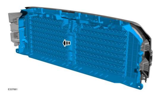
8. If equipped, remove the pin-type retainers and the wire harness.
