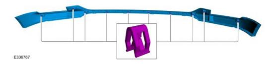
5. Remove the bolts and the pin-type retainer. *Torque*: 36 lb.in (4.1 Nm)
