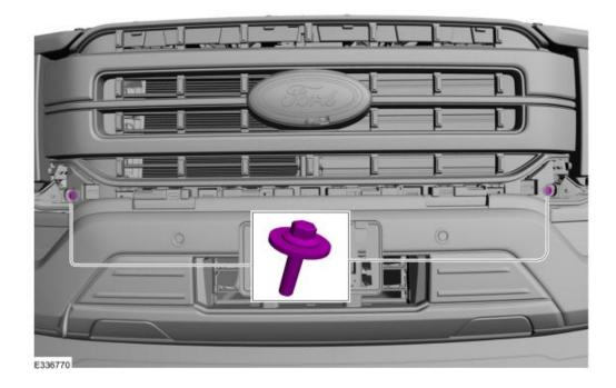
7. Remove the pin-type retainer. Pull up to disengage the locating pins along the top of the grille. Pull forward on center of the grille to remove.
