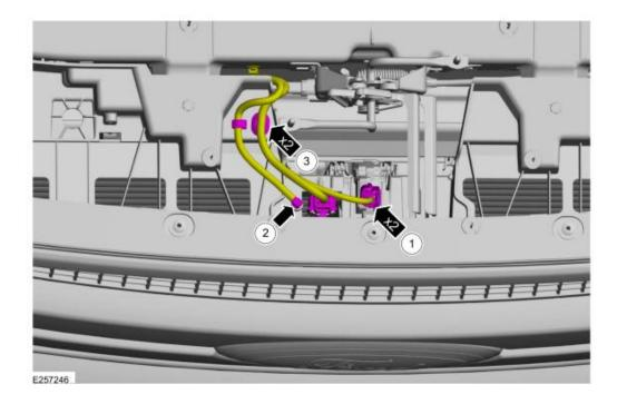
3. On both sides, remove the 2 screws. Torque: 15 lb.in (1.7 Nm)
