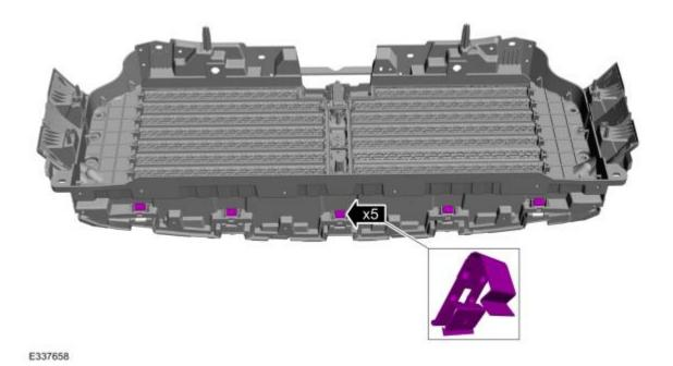
4. Remove the screw and the nuts. *Torque*: 1: 22 lb.in (2.5 Nm) 2: 44 lb.in (5 Nm)
