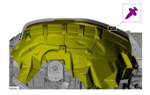
**Step 4:** Remove the screws and the fender splash shield. *Torque*: 15 lb.in (1.7 Nm)
