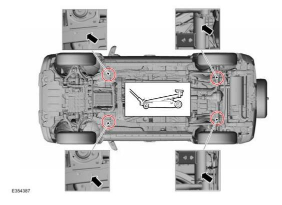
Only the specified jacking points may be used for jacking and supporting the vehicle.
