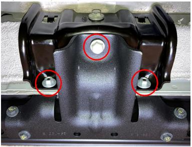
5. On the front of the hoop step assemby, use a M10x20 bolt and 2 M6 nut & washers to secure the hoop step assembly.
