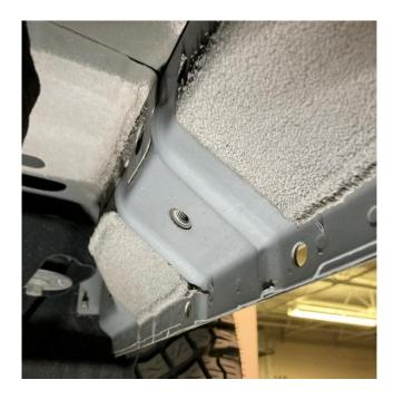
2. Using a M10x20 bolt, secure hoop step bracket to the side of the vehicle. Torque: 18 lb.ft (25 Nm)
