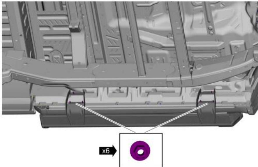
3. Remove the running board assembly.
