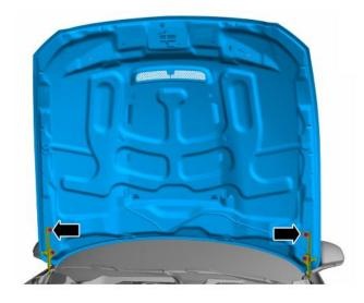
Step 2. Install upper left and right hood hinge strut mount as shown in below photos. Left and right bracket are mirror opposites of each other and fit into the upper hood hinge.
