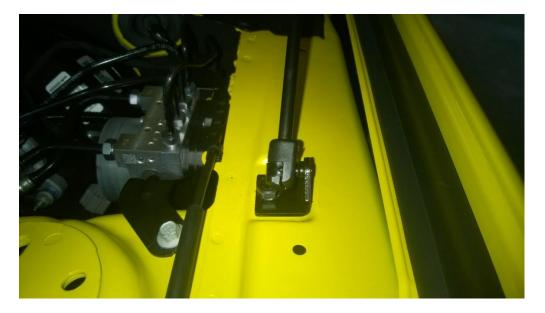
Postion the brackets by putting the bracket retainer inside oval fender hole.
