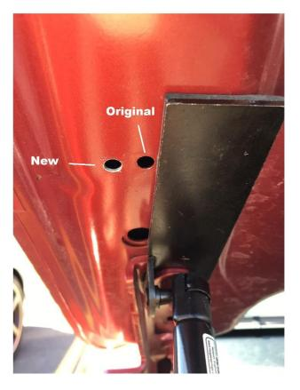
Step 4. Ensure padded part of brackets face straight forward Tighten the nuts to secure the bracket and hood hinge. Torque: 17 lb ft (23 Nm)
