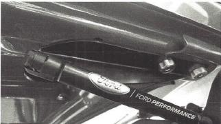
7. Reinstall the forward bolt through the Hood Bracket and thread into hood. Tighten both hood bolts to 106 in. lbs. (approx 9 ft. lbs.) torque spec. Repeat the same steps on the other side.
