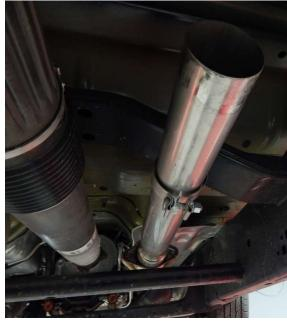
STEP 2: Slide a 3" clamp onto the front pipe. Work the overaxle pipes of the muffler assy over the rear axle, then slide the expanded muffler inlet over the front pipe. Push the hangers into the rubber isolators. Slide the clamp onto the joint, do not tighten.
