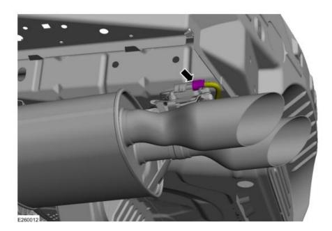
17. **NOTE:** Make sure the electrical wiring is routed with suitable clearance from the exhaust tips and the push pin clips are correctly installed.
