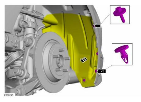
On both sides. Remove the bumper cover to bracket screws. Save for later *Torque*: 18 lb.in (2 Nm)
