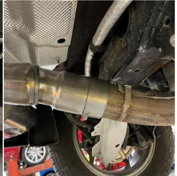
**Step 3:** Place (2) hangers into the rubber isolators.
