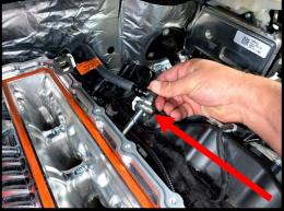
76. Slide the EECPV to previously installed bracket. Connect factory plastic quick connect fitting to EECPV until it clicks and locks into place. Connect 2-way electrical connector to EECPV, press locking tab back in place.
