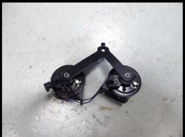
90. Reinstall new horn bracket and horns to factory location, using factory nut. Torque to 106 lbs-in. Zip-tie wire to factory harness for clean installation.
