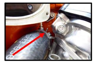
32. (Dual Alternator) Release the (3) factory clamps from thermostat housing coolant lines. Pull hoses away.
