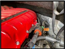
74. Connect the factory high pressure **RH** side rail fitting to the DI pump factory hose, press until it clicks and locks in place. *NOTE: THIS FUEL LINE HAS A CHECK VALVE, NEVER FLIP ORIENTATION FROM STOCK DIRECTION.*
