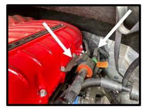
77. Install the supplied 3/8" ID x 13" with 55deg quick connect fitting hose to the EECPV barb fitting and **upper** quick connect fitting on SC inlet. Push until it clicks and locks into place.
