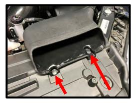
102. Install the supplied panel filter to the airbox lower. Install the upper airbox to the top of the filter. Secure the top to bottom using the supplied (6) 6mm x 16mm BHCS. Torque to 50 in-lbs. \*Caution: Over torquing can result in pulling an insert out of plastic box.
