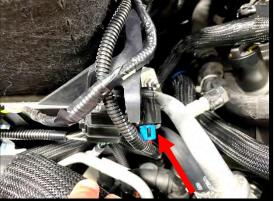
108. Using a 10mm socket, remove the nut on the power stud, located on the positive stud under fuse box cover. Install the IC pump relay power eyelet (red wire) to the power stud on the battery positive (+) stud. Use a 10mm socket to secure stock and IC power wire.
