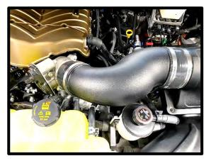
105. Install the stock make up air hose to air tube fitting previously installed. Fittings may require some rotation to properly fit.
