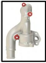
40. (**Dual Alternator**) Install the supplied #2-113 oring to new coolant tube. Install tube to thermostat housing. Secure coolant tube using the (2) 6mm x 50mm HHFCS bolts supplied. Torque all (5) thermostat housing bolts to 89 lbs-in.
