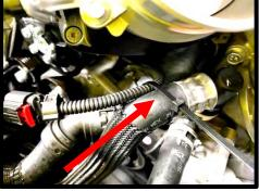
71. Reinstall the water pump pulley using a 10mm socket, torque to 14 lbs-ft.
