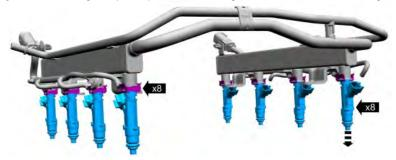
25. Using cutters, remove the clips that secure the injector harness to fuel rail. These clips will not be reused.
