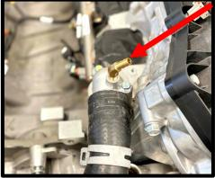
31. (Single Alternator) Reinstall water neck hose to new water neck. Using needle nose pliers, reinstall and rotate the factory pinch clamp at the water neck towards the driver side for future clearance of the SC. NOTE: Image shows clamp with SC installed to illustrate max clearance.
