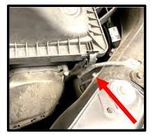
101. Install the supplied lower airbox into factory (2) hole locations. Using the supplied (2) 1.1" L x .30" W plastic push pins, secure front of snorkel to factory location.
