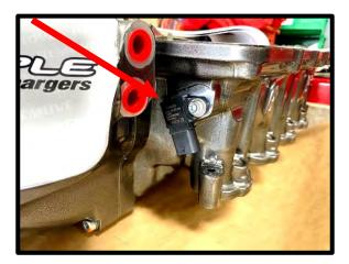
60. Install the supplied TMAP pigtail to the 3-Bar TMAP supplied, wrap up to SC inlet as this will get connected to stock harness later.
