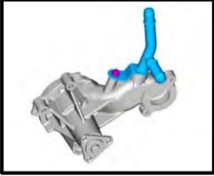
29. (Single Alternator) Install the supplied #2-113 oring to the shorter heater tube and install to factory location, secure with stock fastener, torque to 89 lbs-in. Reconnect both factory hoses, secure lower hose with stock clamp. NOTE: Some 2022 models, built without the auto start/stop pump are equipped with a 55deg fitting. Remove the stock fitting from stock hose, install the supplied 90deg fitting, secure with stock clamp.
