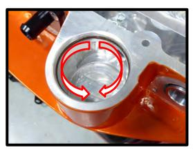
73. Apply generous amount of grease to the (1) #2-230 Viton bypass oring. Install the supercharger lid to the supercharger housing by carefully placing the bypass down. Secure the SC lid using the (17) 6mm x 30mm HHFCS and (3) 6mm x 90mm HHFCS (*marked green*) using the following pattern. Slide the EECPV bracket under bolts 3 and 5 from image (bank 2). Torque to 90 lbs-in using an 10mm socket.
