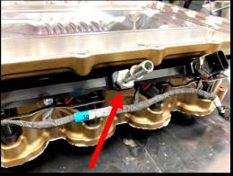
51. Install the supplied (1) #2-906 Viton oring to the (1 of 2) 45mm long 9.49mm outlet fitting. Apply light amount of grease to oring for ease of installation, install to rail.
