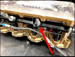
50. Install the supplied (1) #2-906 Viton oring to the (1 of 2) 45mm long 9.49mm inlet fitting to fuel rail. Apply light amount of grease to oring for ease of installation, install to rail.
