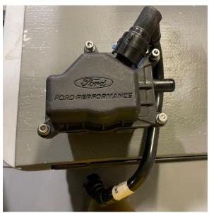
Install oil separator on the bracket and then install LH inlet tube from engine to oil separator.
