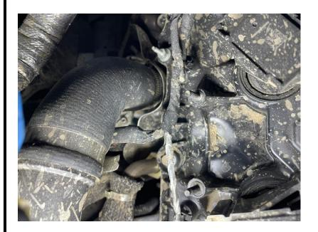
For the RH (passenger's) side, find the threaded studs on the RH camcover. Intall the RH oil separator bracket onto the studs using W520201-S440 nuts and torque to 10Nm (88 lbin).
