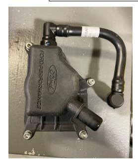
Install oil separator on the bracket and then install RH inlet tube from engine to oil separator.
