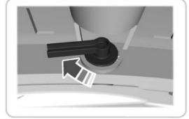
2. Lock the five quarter turn clips by turning the clips clockwise.
